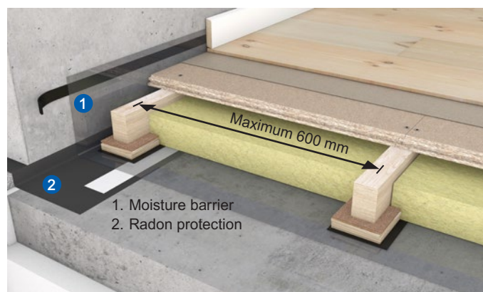
Figure 1 Subfloors on ground floors should always have a moisture barrier and radon barrier on the concrete surface.
